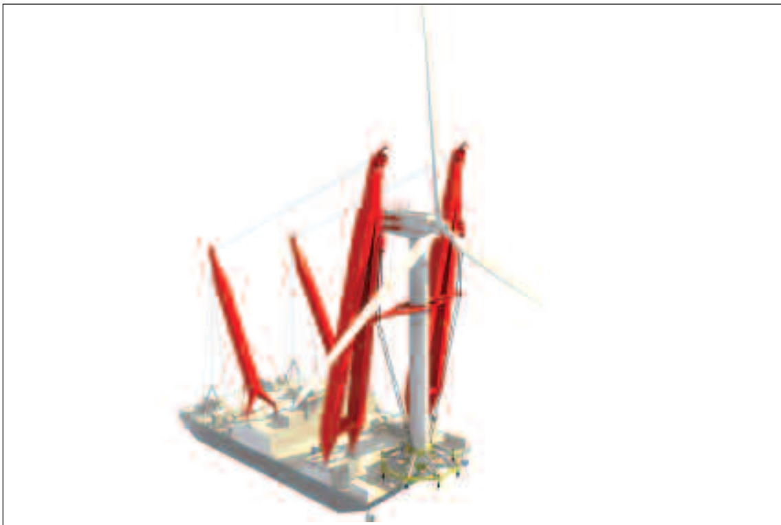
Figure 7.1 Tower and turbine ready for transportation.
